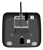
To disconnect the plug from the charger, press the release button **1** and disconnect the plug **2**.
