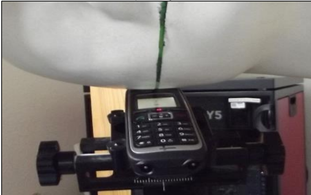
Photo 15: Test position right hand tilted 15°
