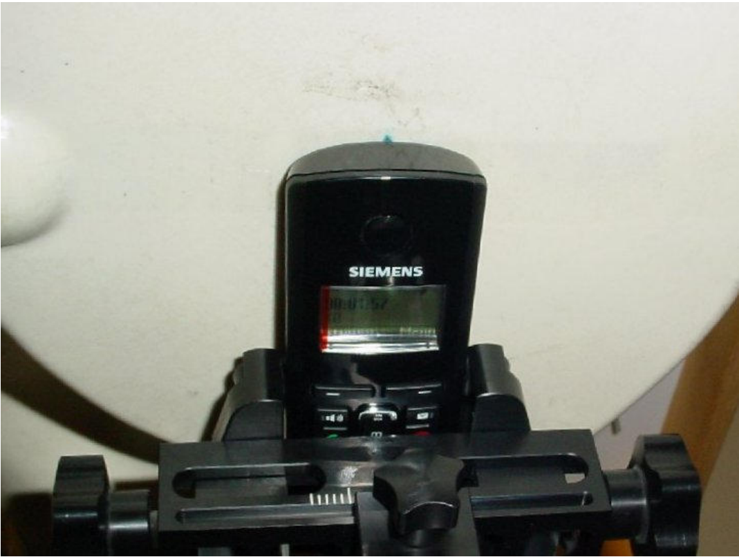
Photo 19: Test position body worn rear side without any distance
