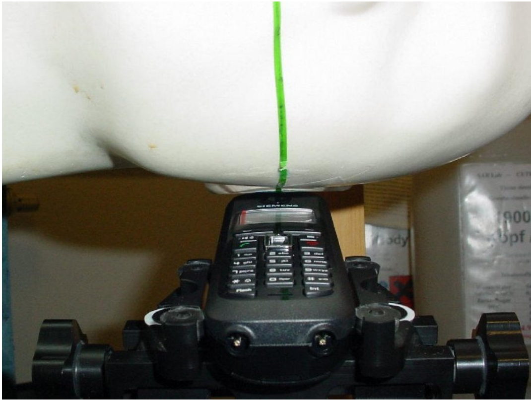
Photo 10: Test position left hand tilted 15°
