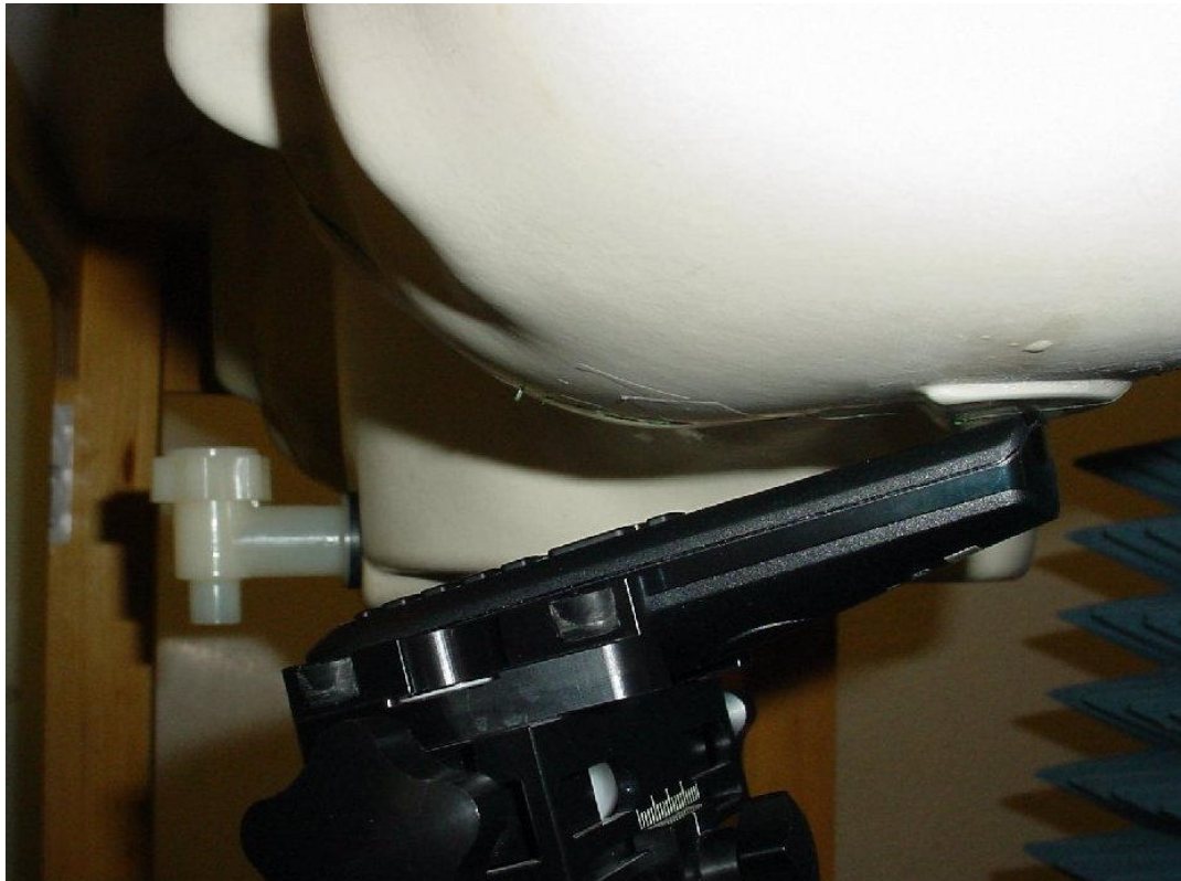
Photo 10: Test position left hand tilted 15°
