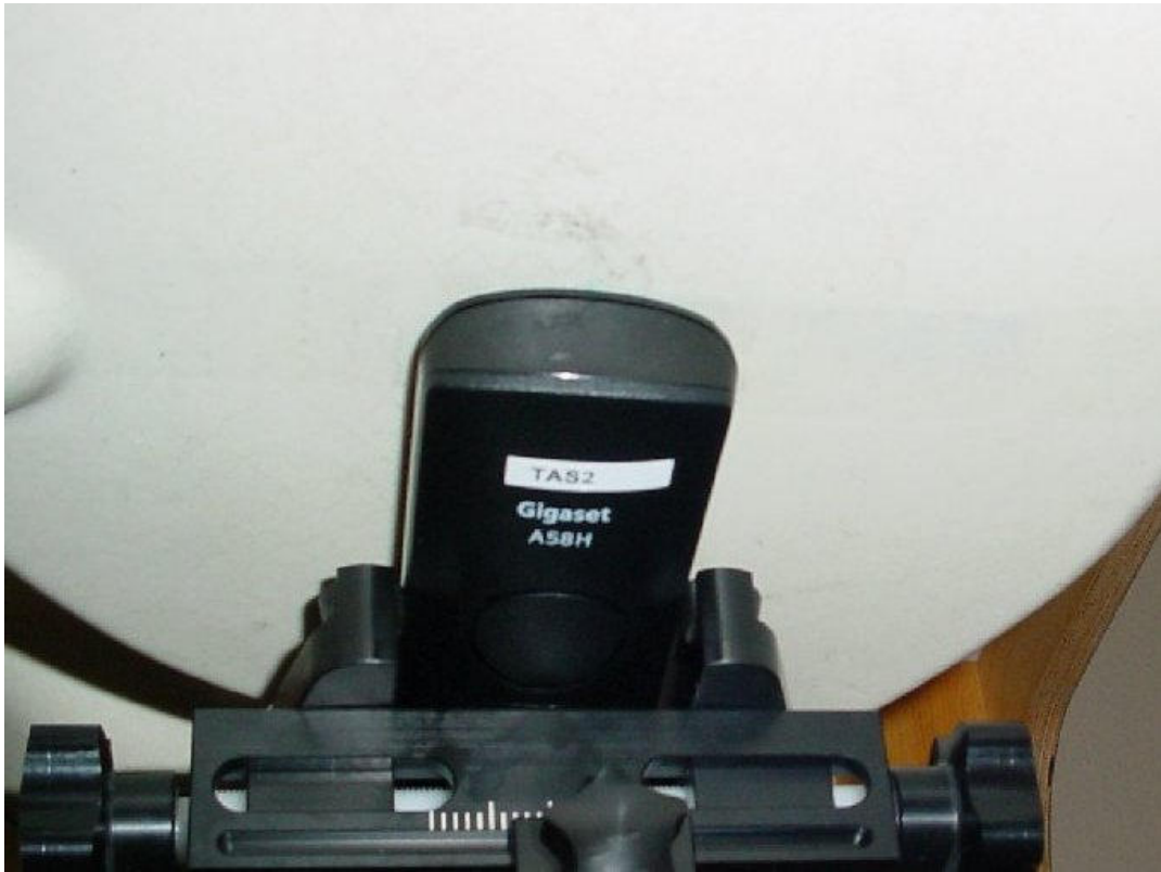
Photo 18: Test position body worn rear side without any distance
