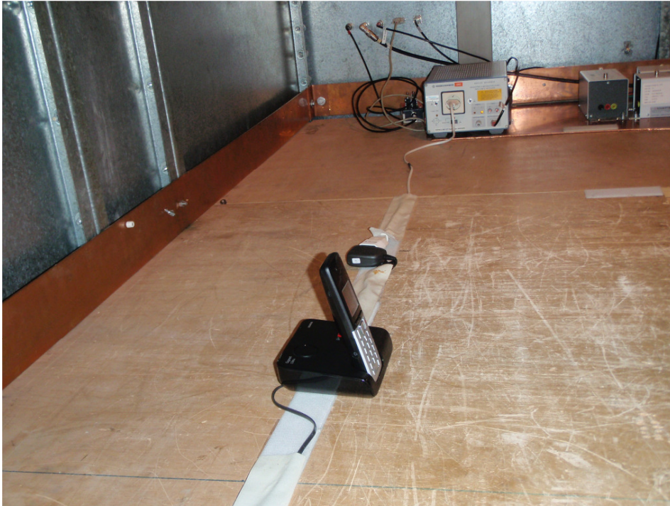
Photo 1: Power Line Conducted Emission Test
