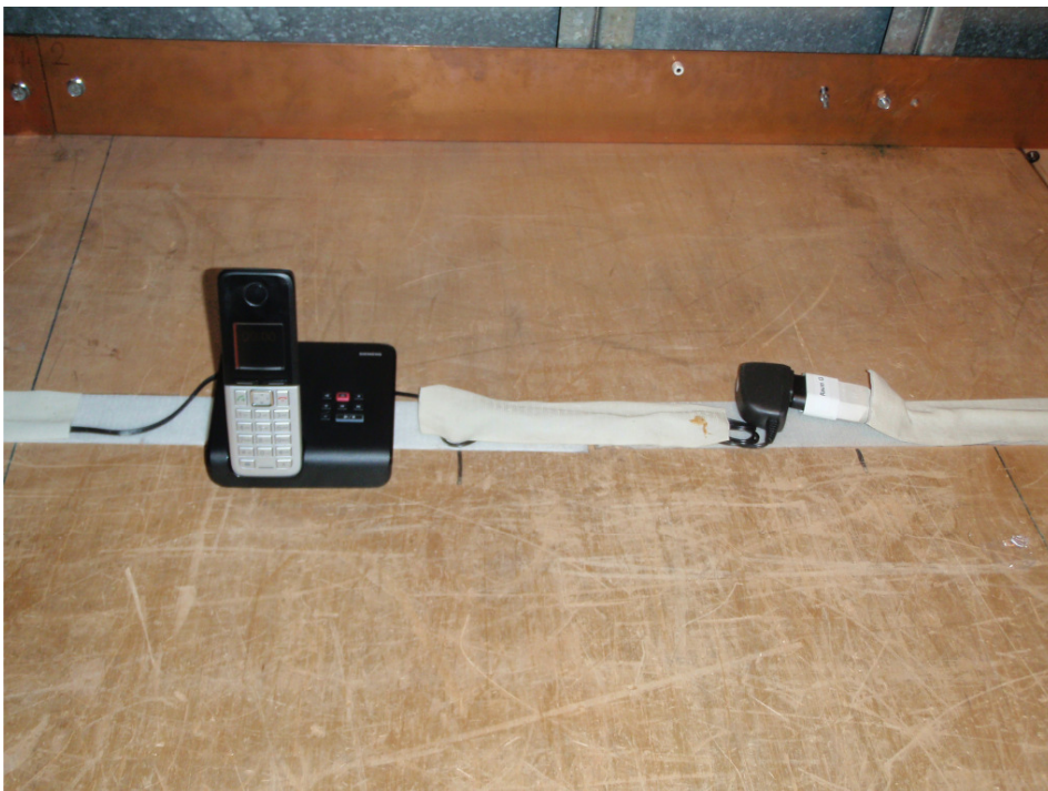
Photo 2: Power Line Conducted Emission Test
