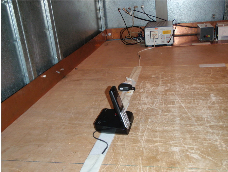
Photo 1: Power Line Conducted Emission Test
