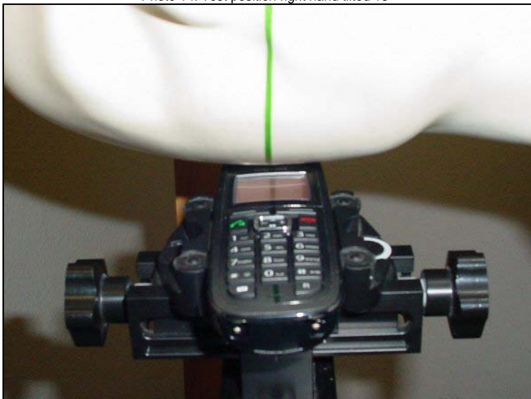
Photo 14: Test position right hand tilted 15°
