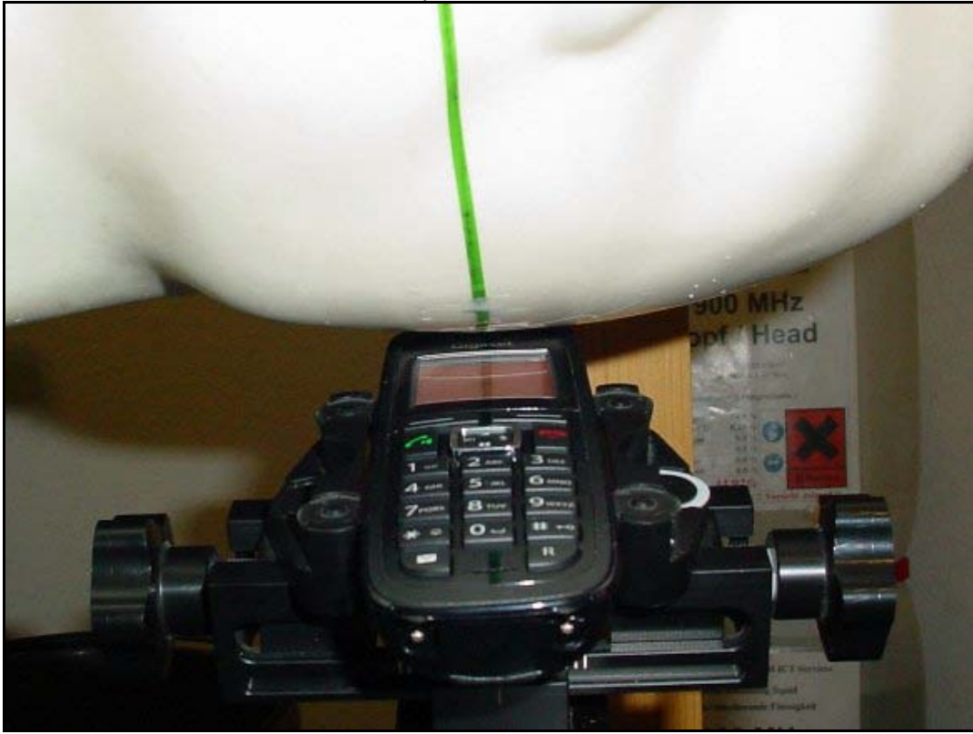
Photo 10: Test position left hand tilted 15°
