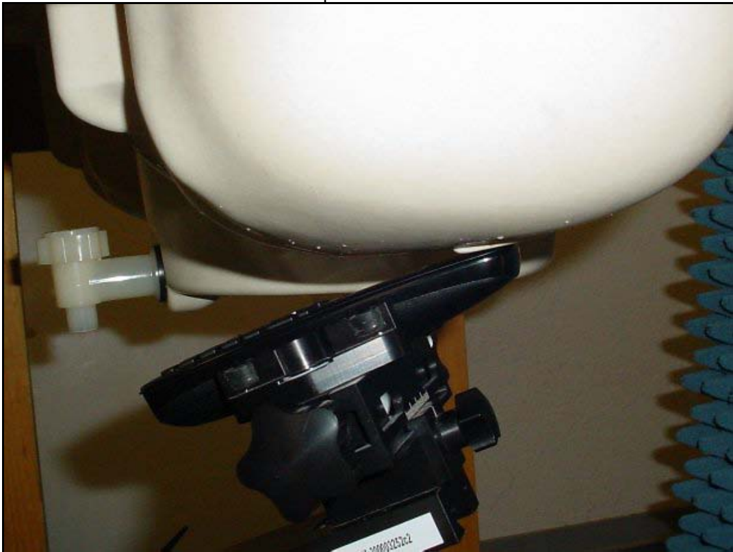
Photo 10: Test position left hand tilted 15°
