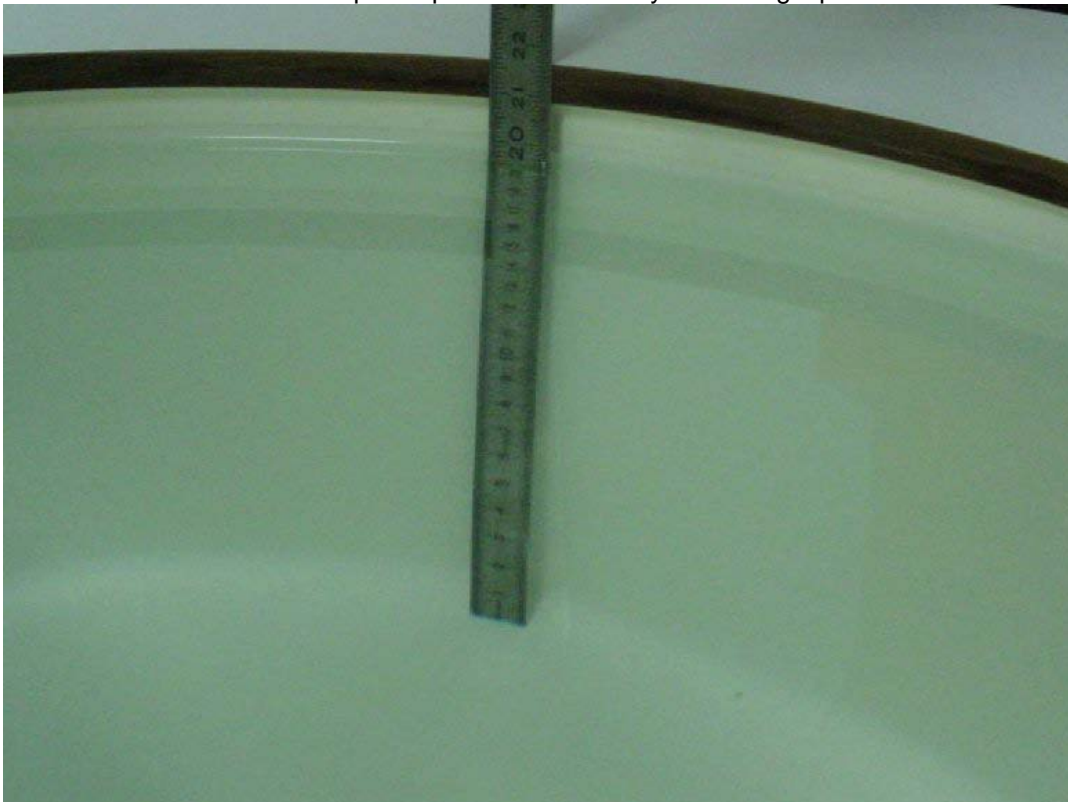
Photo 2: Liquid depth 1900 MHz body simulating liquid
