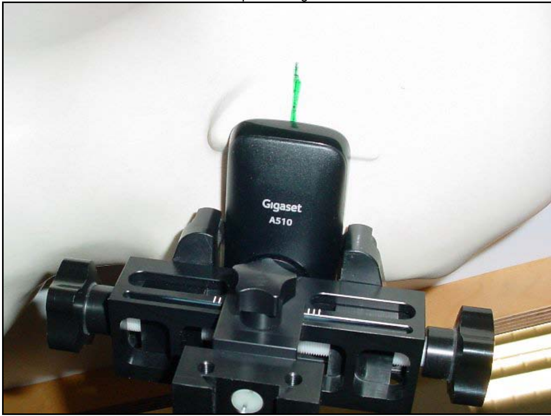
Photo 14: Test position right hand tilted 15°
