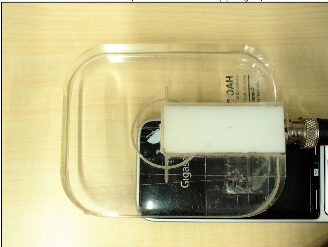
Photo 4: test setup for Radial field intensity (0 degree)
