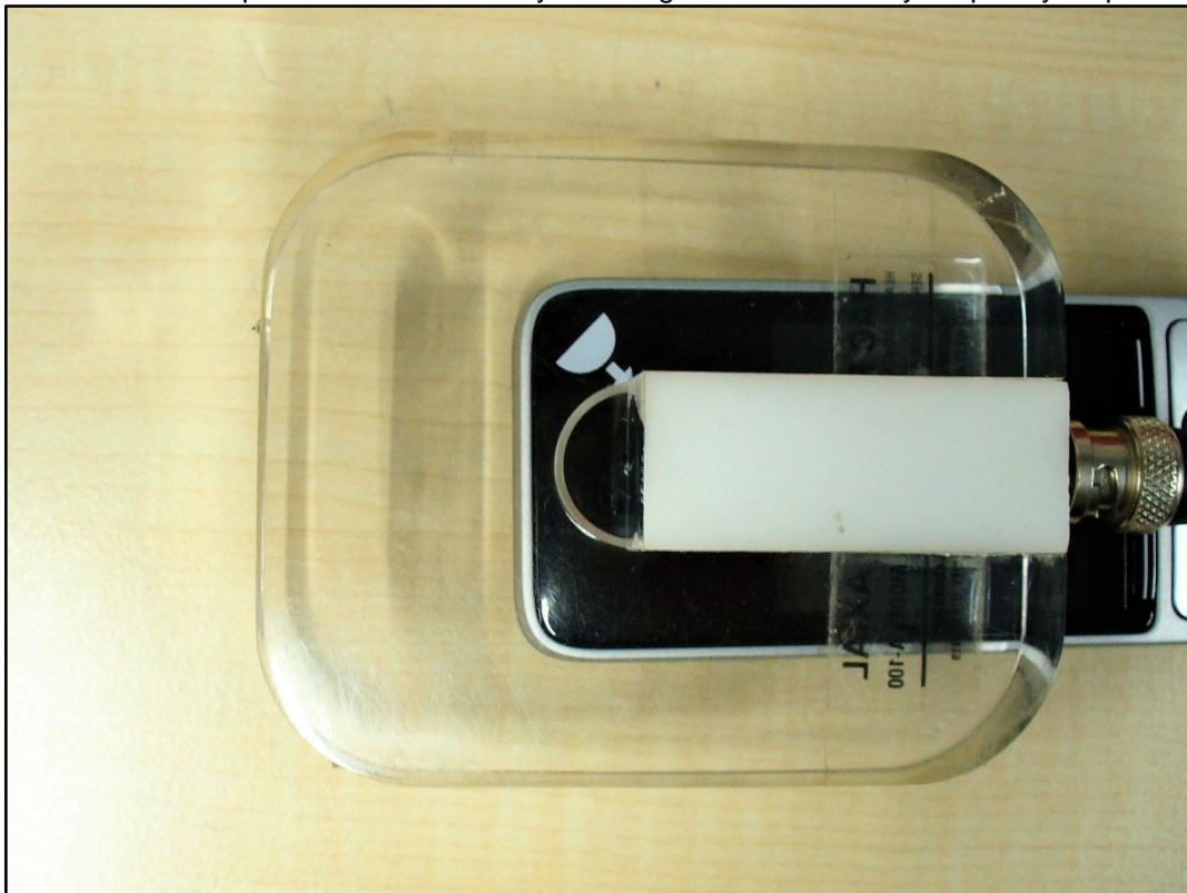
Photo 4: test setup for Radial field intensity (0 degree)
