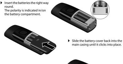
If you need to open the battery cover, for instance to replace the batteries, place your fingertip in the grooved area on the top of the cover and slide down.
