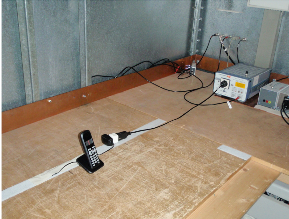
Photo 1: Power Line Conducted Emission Test
