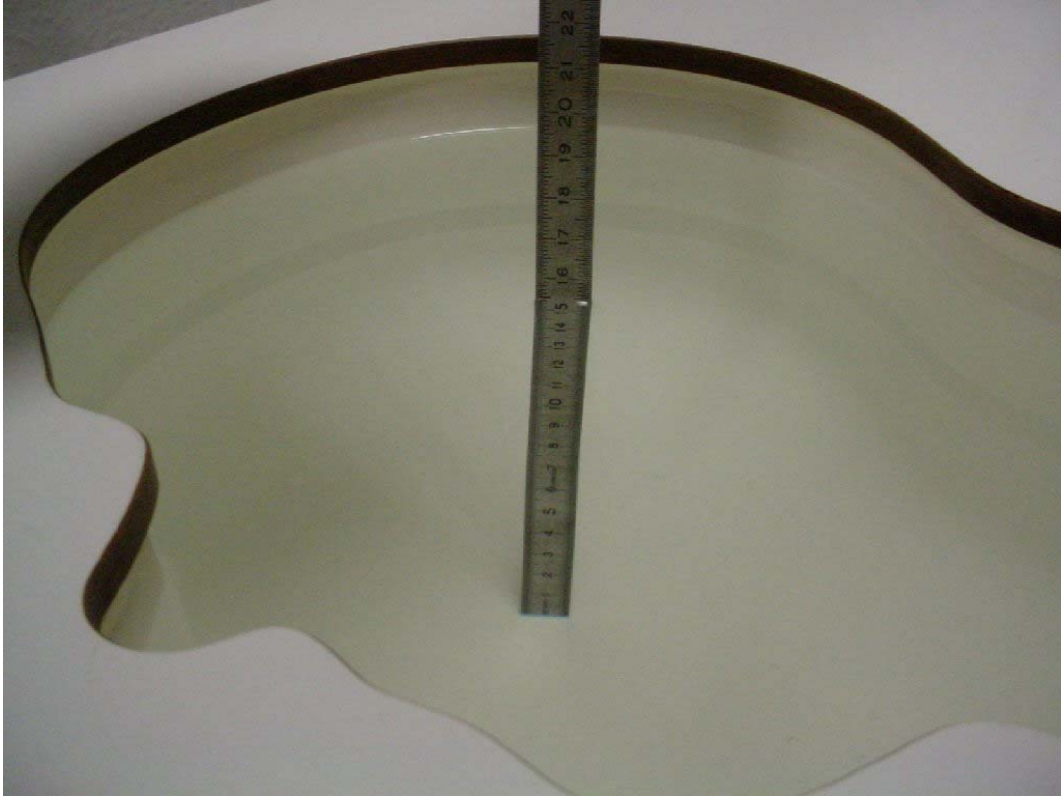
Photo 2: Liquid depth 1900 MHz body simulating liquid
