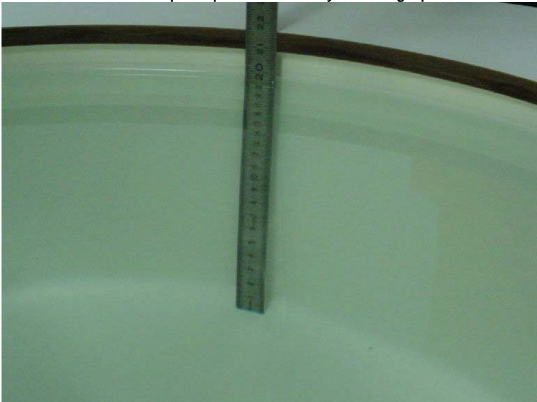
Photo 2: Liquid depth 1900 MHz body simulating liquid
