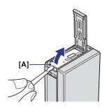
4 Insert a flat-bladed screwdriver, etc., into the "Memory Stick Duo" slot and lift the cover up in the direction of the arrow.
