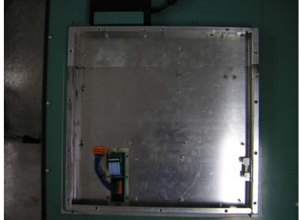
Diplexer Shielding Enclosure
