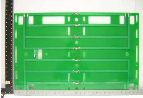
Right Side Inner Antenna Front
