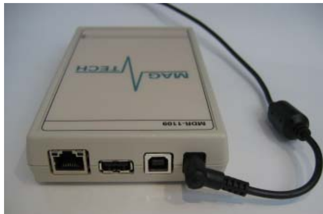
MDR-1109 with plugged-in low voltage power cable
