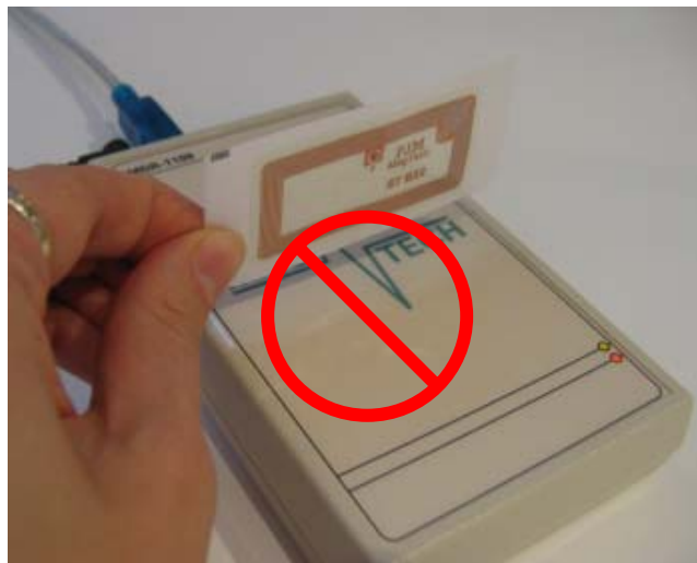
Incorrect orientation (90° angle).
