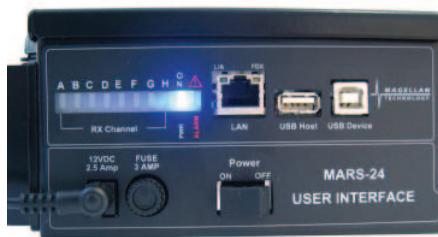
MARS-24E with the blue LED. The Reader is in an operational mode
