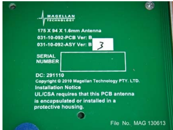
Loop Antenna Labelling Detail
