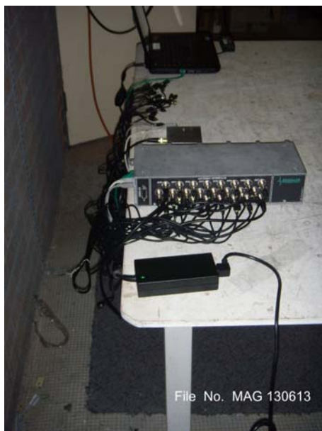
Conducted Disturbance (Dummy Load) Test Setup
