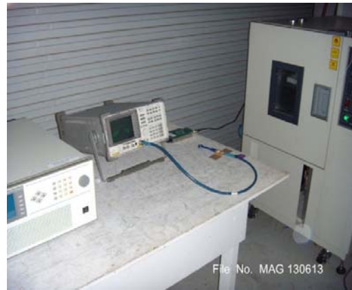
Frequency Stability Test Setup – (15.225)
