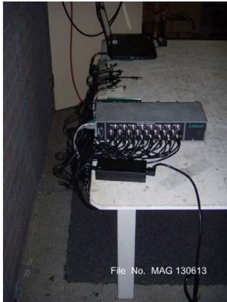
Conducted Disturbance (Antenna) Test Setup
