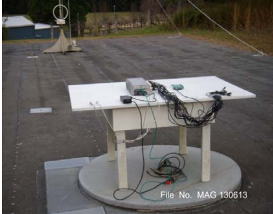
Radiated Disturbance Test Setup – (15.225)
