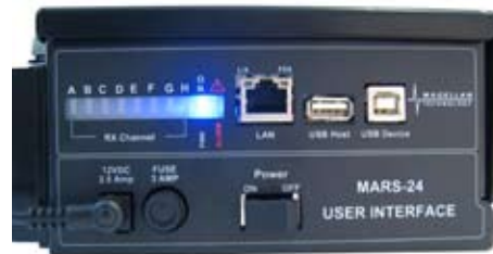
MARS-24AT with the blue LED. The Reader is in an operational mode
