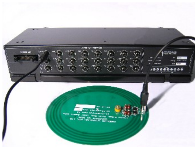
MARS-24 with the external 124 mm diam. antenna connected
