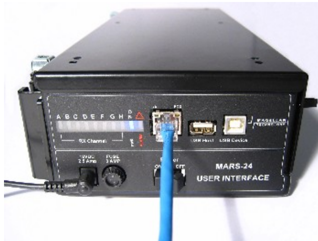
MARS-24 with the Ethernet communication cable and power cable
