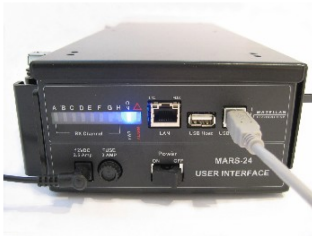
MARS-24 with the USB communication cable and power cable
