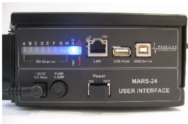
MARS-24 with the blue LED. The Reader is in an operational mode
