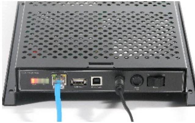
MARS-1 with the Ethernet communication cable and power cable
