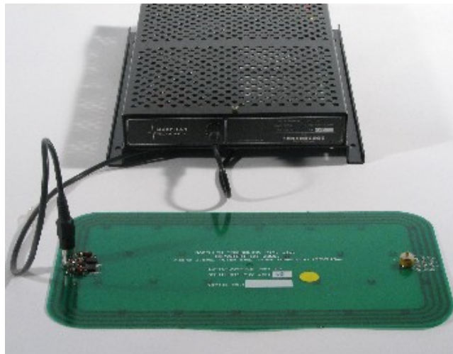
MARS-1 with the external 120x240 mm antenna connected
