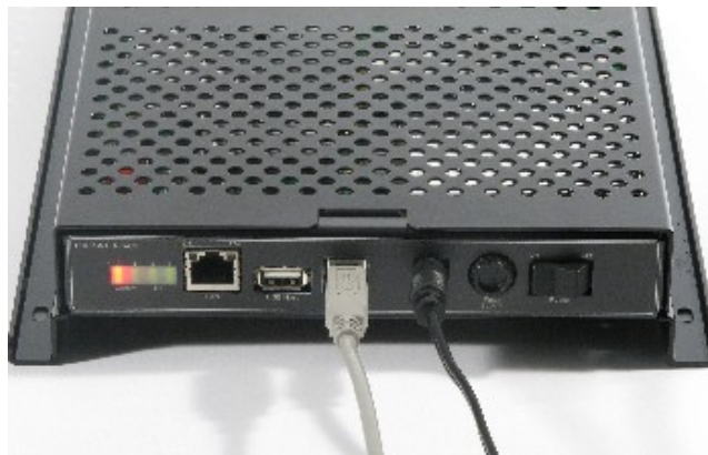
MARS with the USB communication cable and power cable
