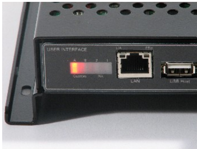
MARS with the red LED. The Reader is in an operational mode
