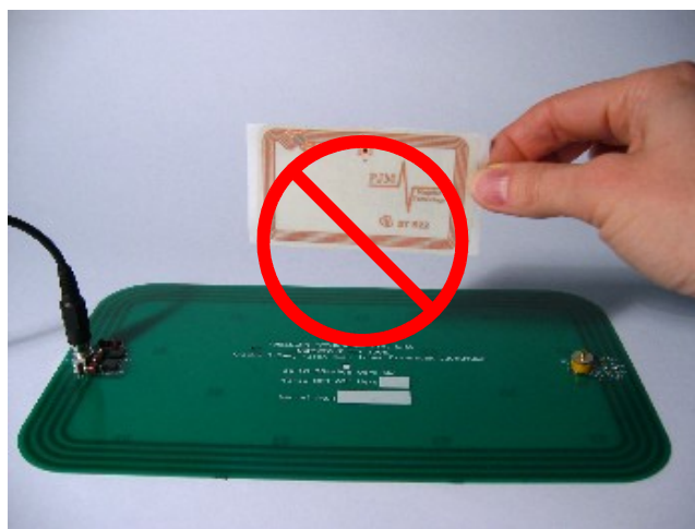
Incorrect orientation (90° angle)
