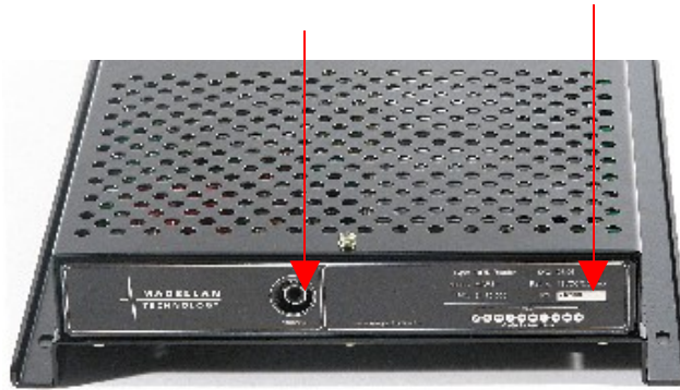
MARS-1 Antenna Interface and OEM label panel
