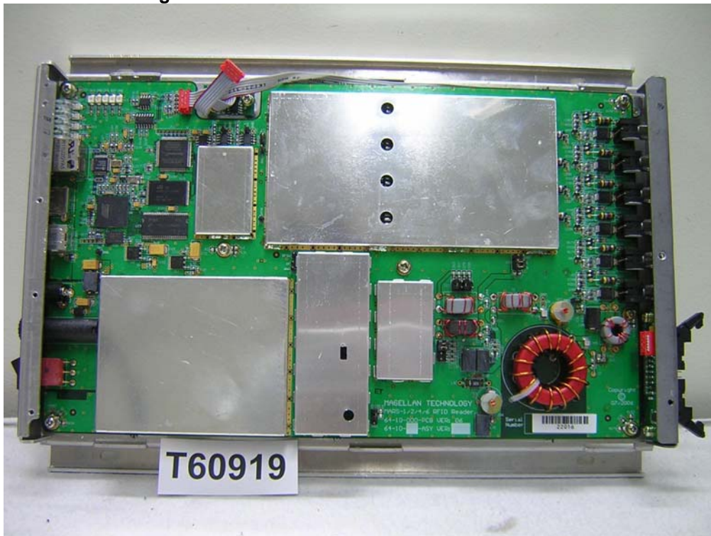
Main Board With Shielding Cans
