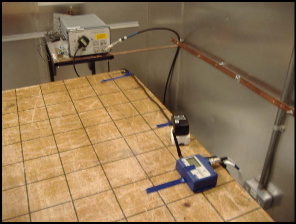
AC POWERLINE CONDUCTION TEST SETUP
