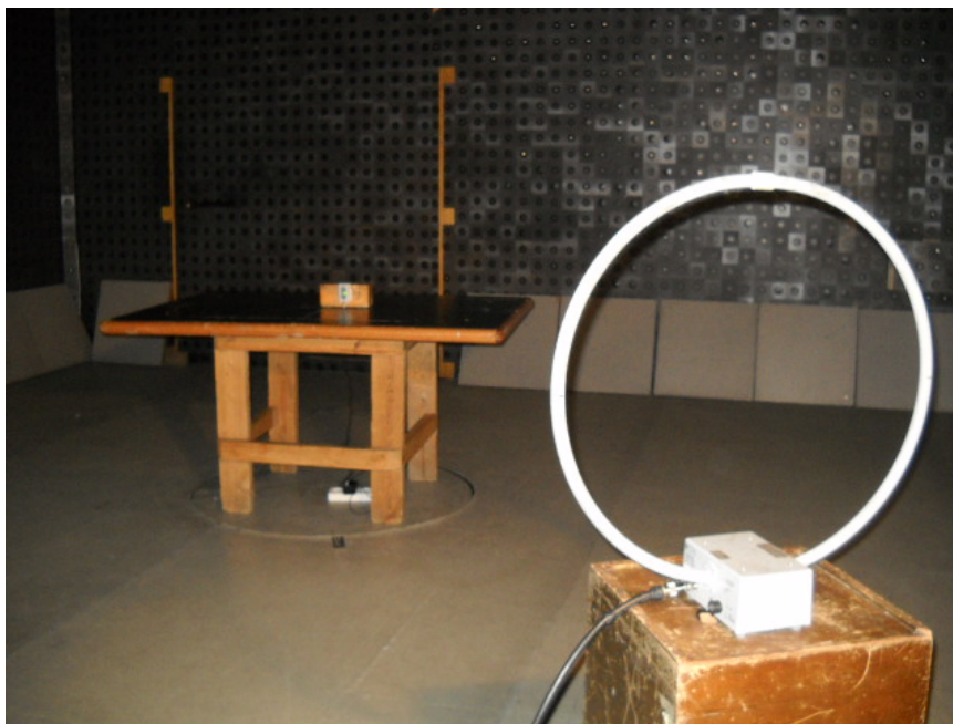
Photograph No.1 Setup for spurious emission field strength measurements below 30 MHz in the anechoic chamber
