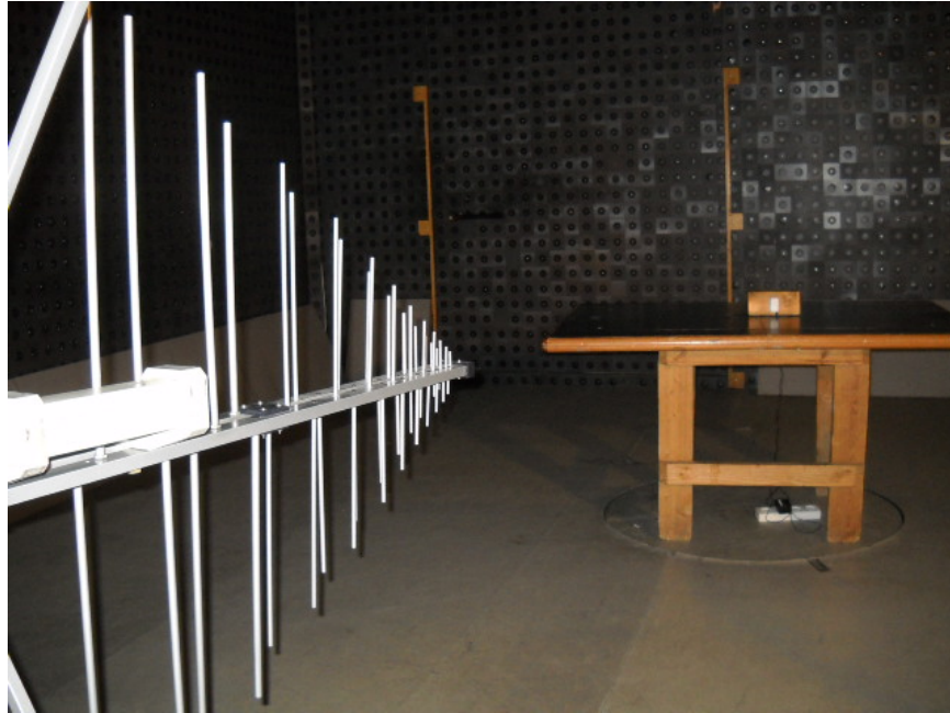
Photograph No.2 Setup for spurious emission field strength measurements from 30 MHz to 1000 MHz in the anechoic chamber
