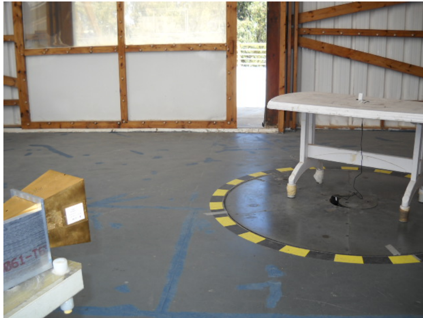
Photograph No.4 Setup for field strength emission measurements at the OATS from 18 to 25 GHz
