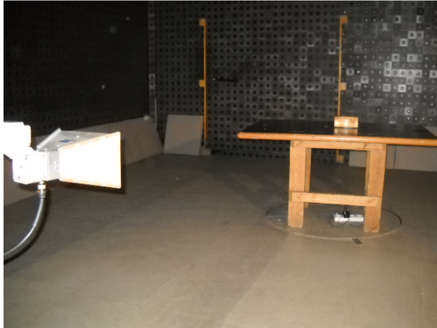
Photograph No.3 Setup for carrier, spurious emission field strength and occupied bandwidth measurements from 1 to 18 GHz in the anechoic chamber
