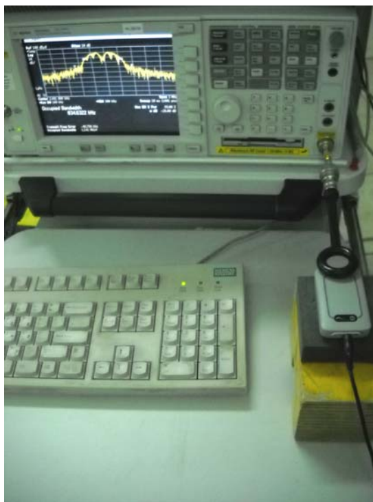
Photograph No.1 Setup for occupied bandwidth measurements
