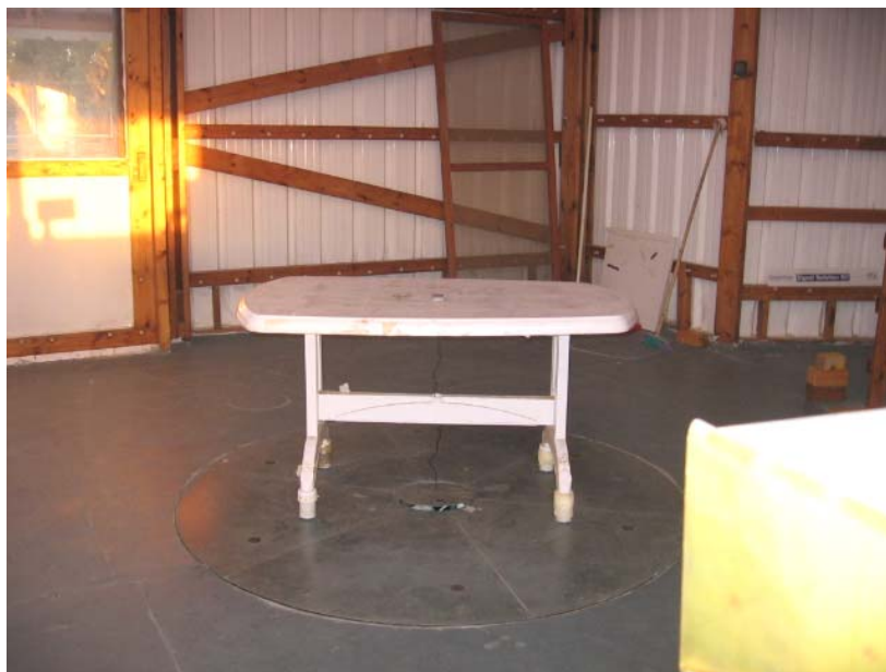
Photograph No.5 Setup for field strength emission measurements at the OATS above 1000 MHz
