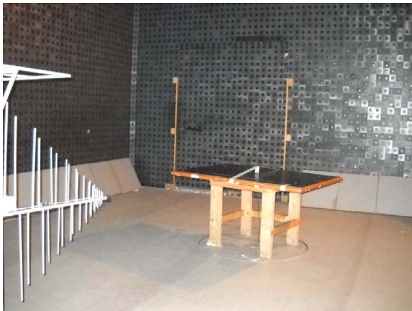
Photograph No.3 Setup for spurious emission field strength measurements from 30 MHz to 1000 MHz in the anechoic chamber
