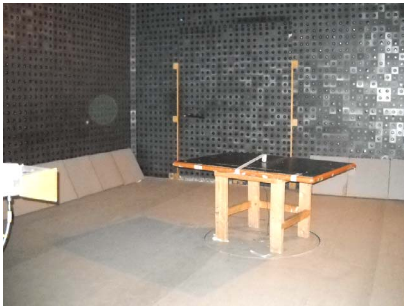
Photograph No.4 Setup for carrier and spurious emission field strength measurements above 1 GHz in the anechoic chamber
