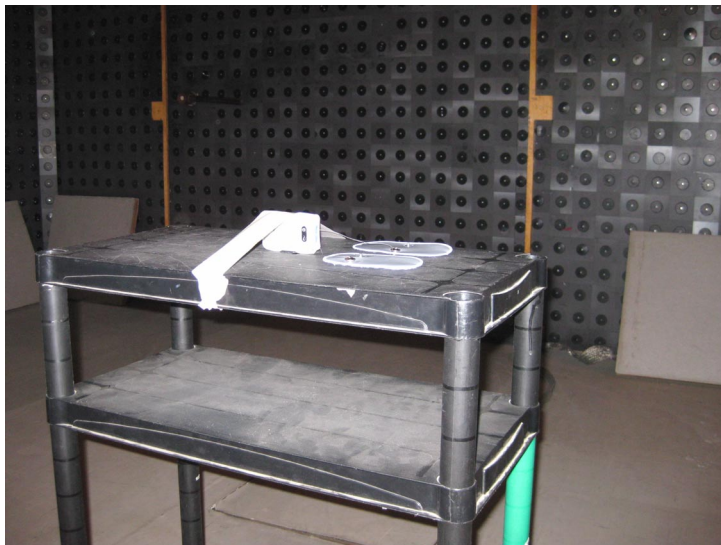
Photograph No.2 Setup for spurious emission field strength measurements in the anechoic chamber, close view
