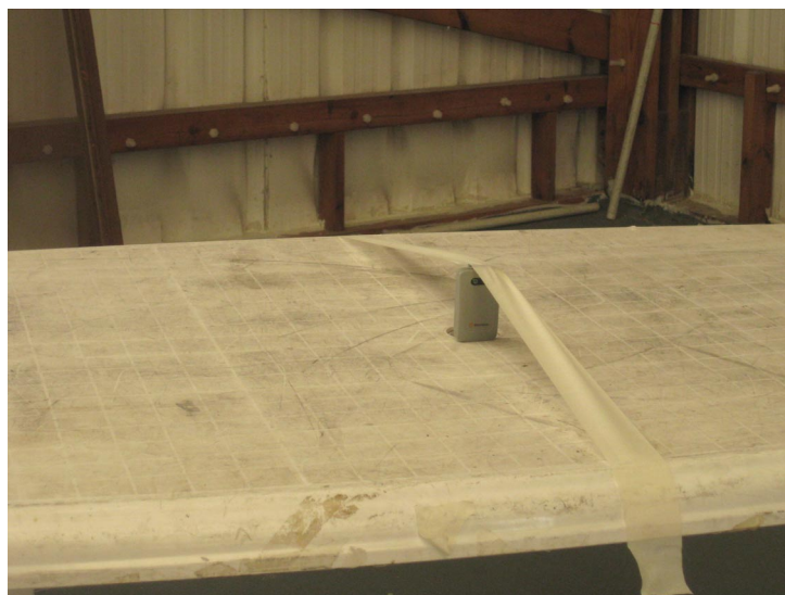
Photograph No.4 Setup for spurious emission measurements at the OATS above 1000 MHz
