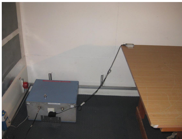
Photograph No.5 Setup for conducted emission measurements on the EUT power lines
