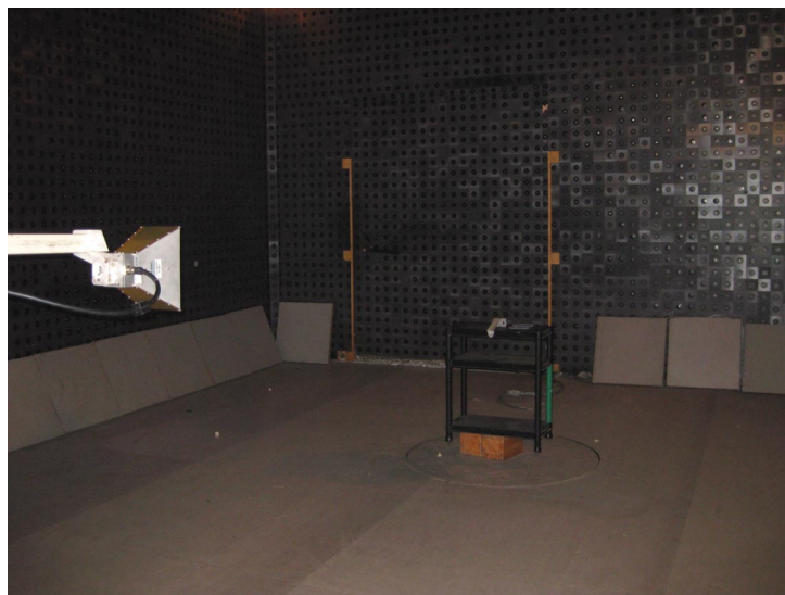
Photograph No.3 Setup for carrier and spurious emission field strength measurements above 1 GHz in the anechoic chamber
