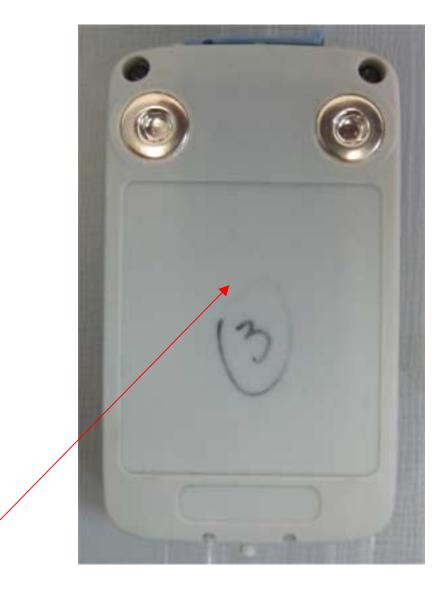
The label shown in the page 1 with FCC ID:TVF-L3P-T-RFS-V10, will be located here. The part 15 statement required by FCC rules, paragraph 15.19 (a)(3), is inserted into the User\_guide\_20763, paragraph "Conformity Certification", page 12, provided to the user together with each unit.
