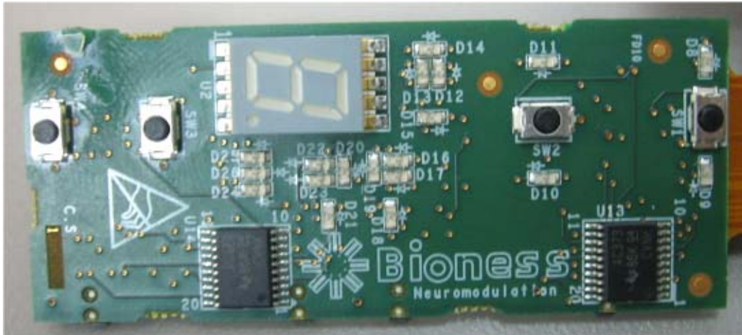
Photograph No.3 Control unit keypad PCB front view
