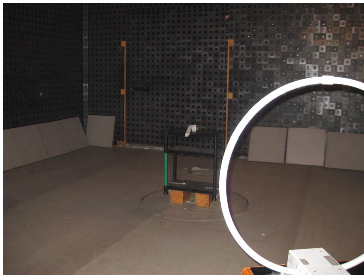
Photograph No.1 Setup for spurious emission field strength measurements below 30 MHz in the anechoic chamber
