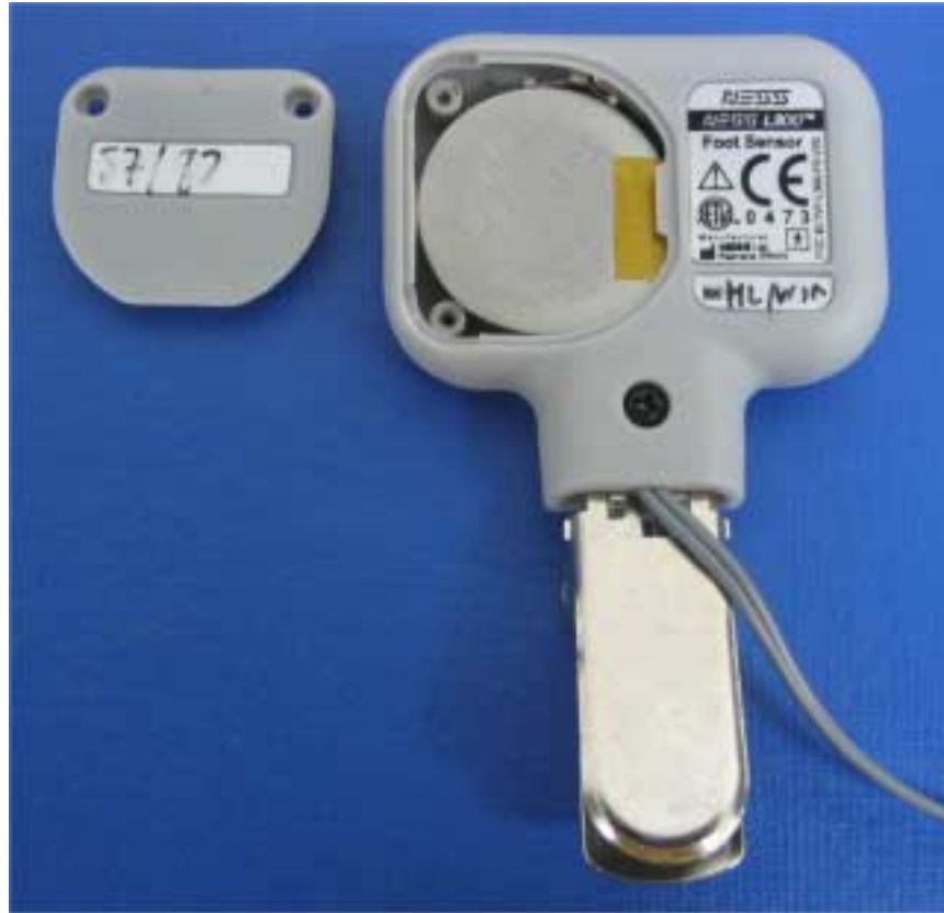
Photograph No.4 Foot sensor (FS) rear side view with battery cover removed
