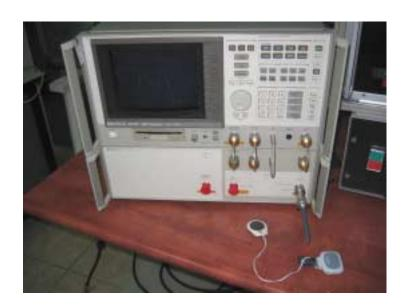
Photograph No.2 Setup for spurious emission field strength measurements in 9 kHz to 30 MHz range
