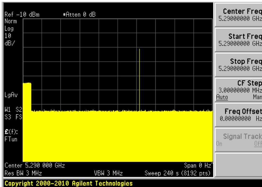
No transmissions found after radar signal applied.
