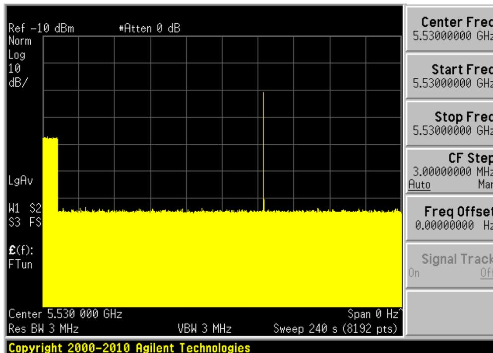
No transmissions found after radar signal applied.
