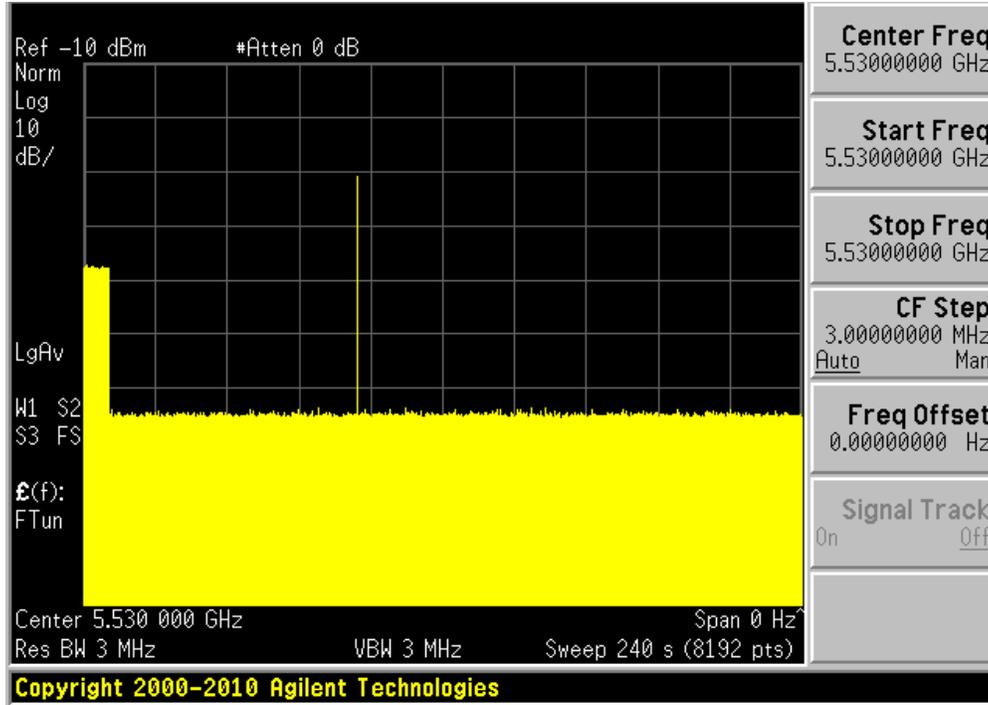
No transmissions found after radar signal applied.
