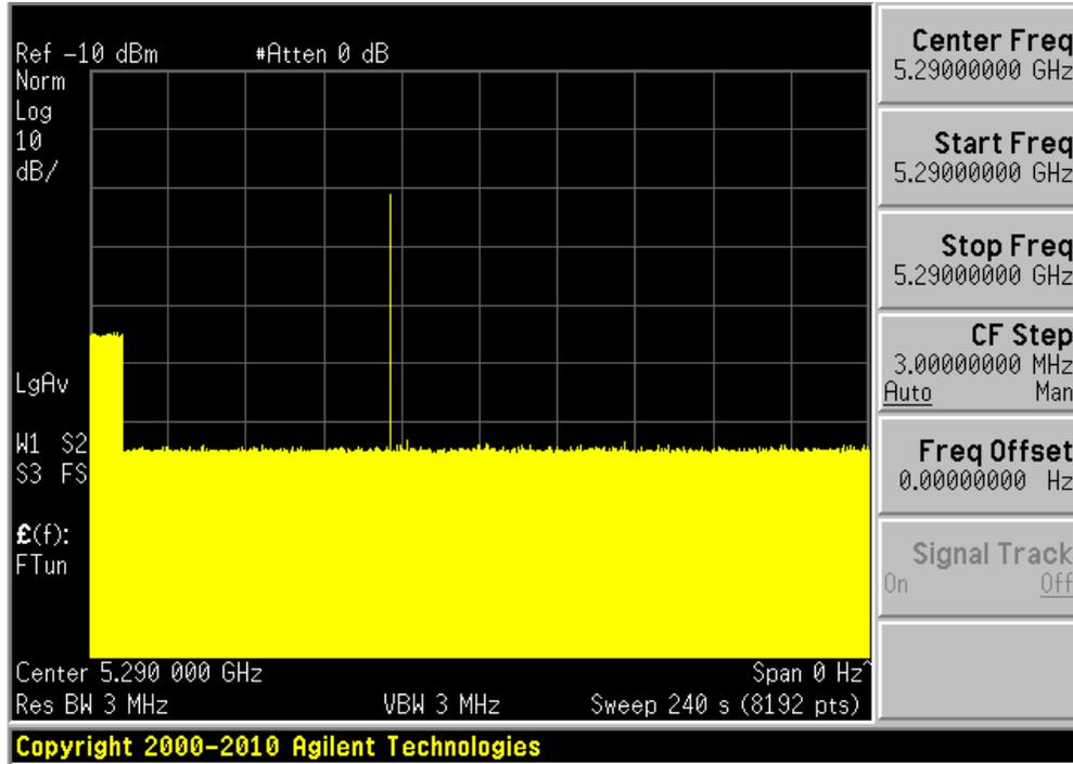
No transmissions found after radar signal applied.
