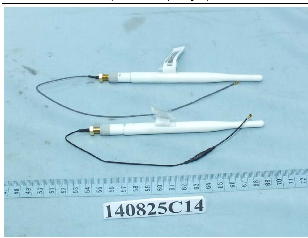
Dipole antenna (3dBi gain)
