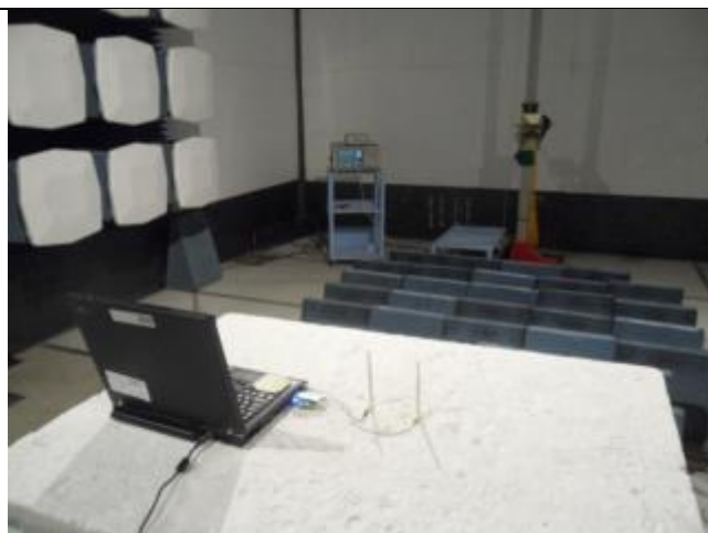
Radiated Emissions (>1GHz) – Rear View (Ext. Antennas)
