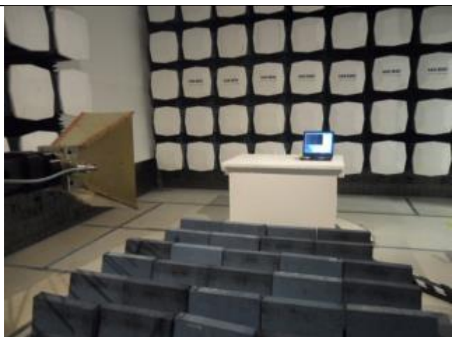
Radiated Emissions (>1GHz) – Front View (Ext. Antennas)
