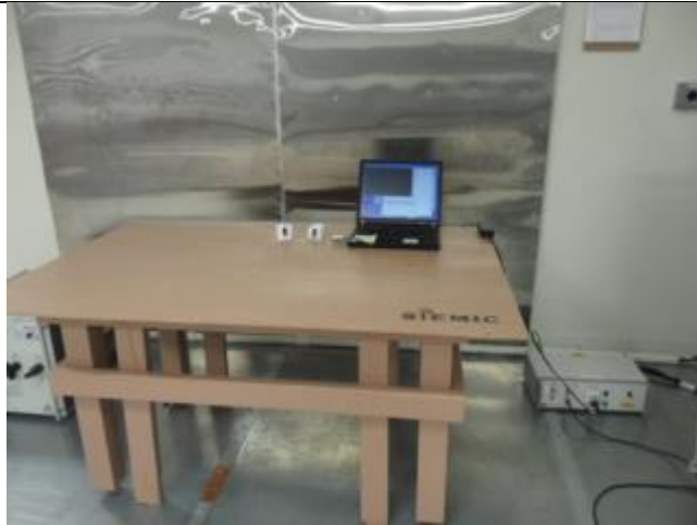
AC Line Conducted Emissions – Front View
