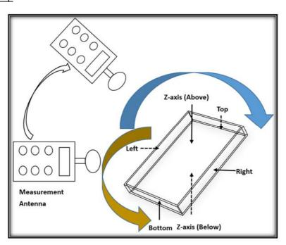
Note: The measurement antenna are move and surrounding the EUT when performed the test, the test results recorded the highest values for each sides of the EUT (left/right/top/bottom/z-axis)
