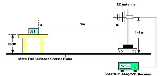
For radiated test from 1GHz to 18GHz
