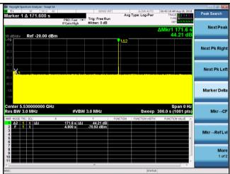
Radar at end of CAC - VHT80 - 5290MHz
