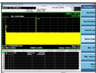
Radar at beginning of CAC - VHT80 - 5290MHz
