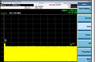
Channel Move Time& Closing Time - 802.11ac-5530MHz (Type0)
