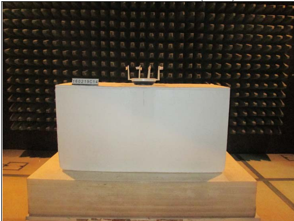
Radiated Emission Test above 1GHz (Mode D)
