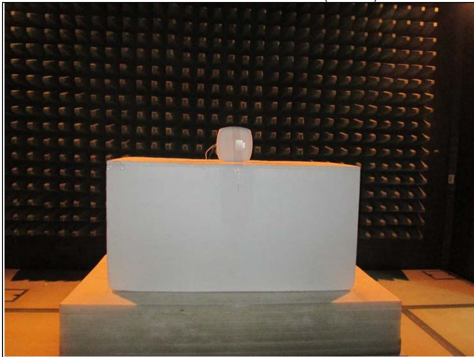
Radiated Emission Test above 1GHz (Mode B)
