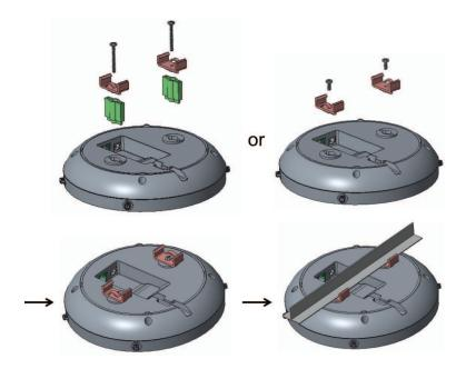
The unit can be mounted on a wall or ceiling using the mounting hardware provided.
