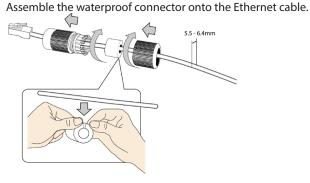
6. Connect the Ethernet cable. The cable can be stored in the EMT tubing or in the hole in the wall or ceiling.
