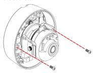
10. Open the MicroSD card socket lid by sliding it backwards. This and the following two steps are only required if onboard storage is preferred.
