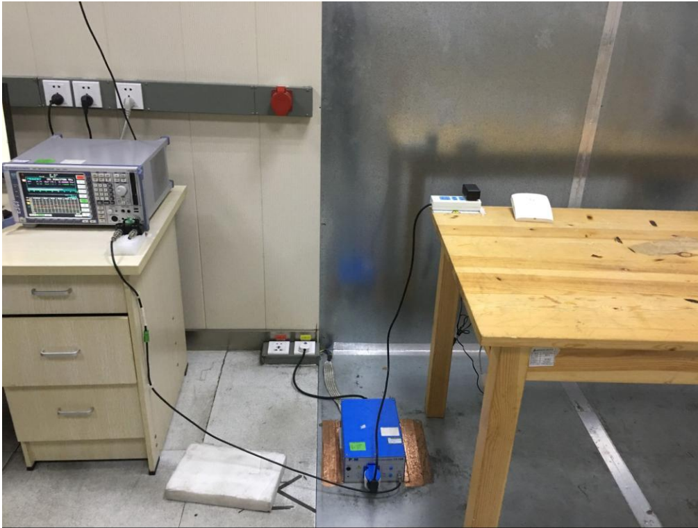
FCC RADIATED EMISSION TEST SETUP BELOW 1GHZ
