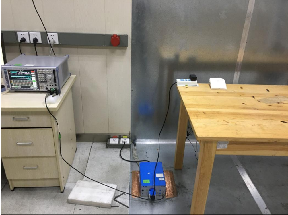
FCC RADIATED EMISSION TEST SETUP BELOW 1GHZ
