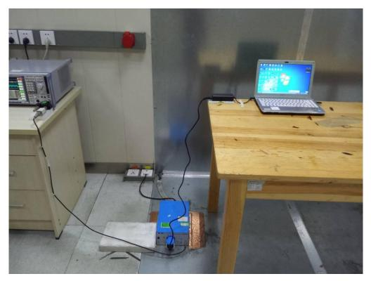
FCC RADIATED EMISSION TEST SETUP BELOW 1GHZ
