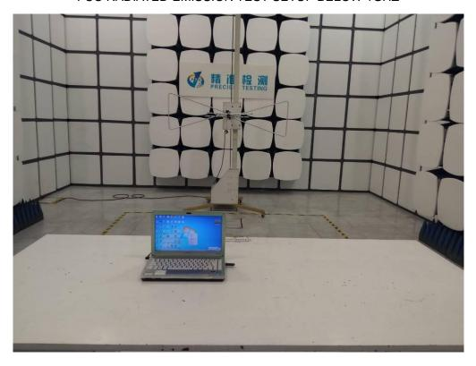
FCC RADIATED EMISSION TEST SETUP ABOVE 1GHZ
