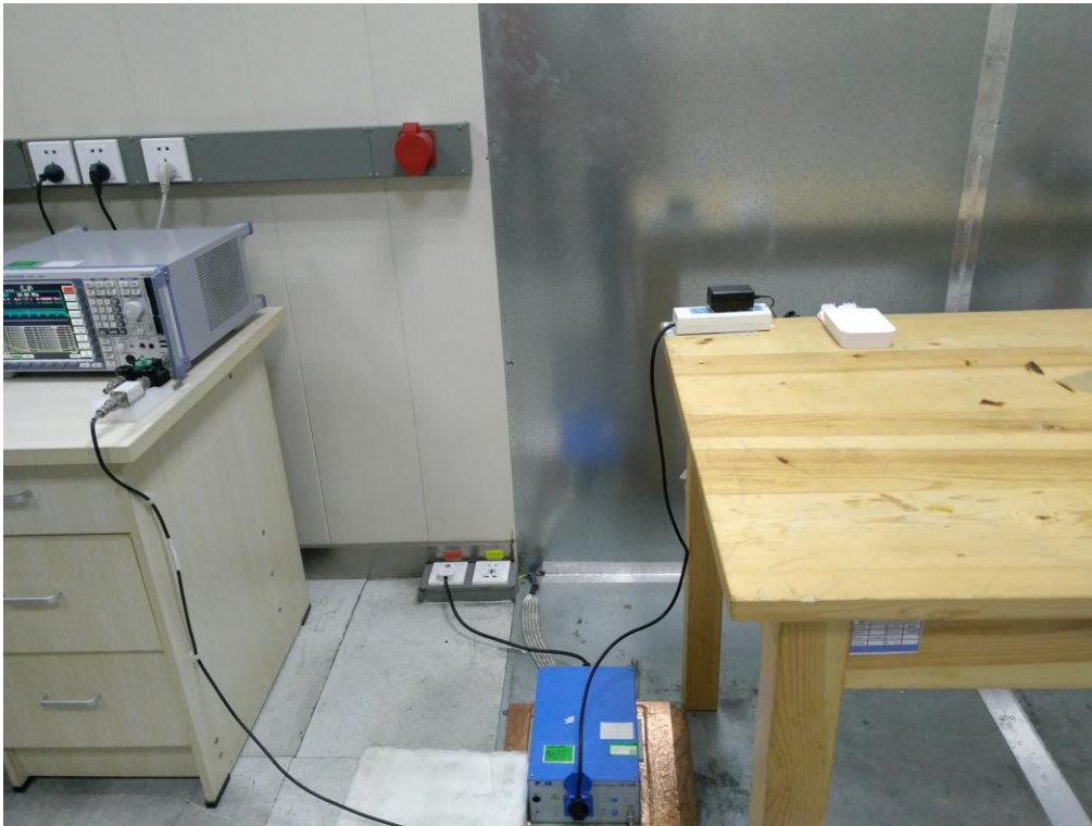
FCC RADIATED EMISSION TEST SETUP BELOW 1GHZ
