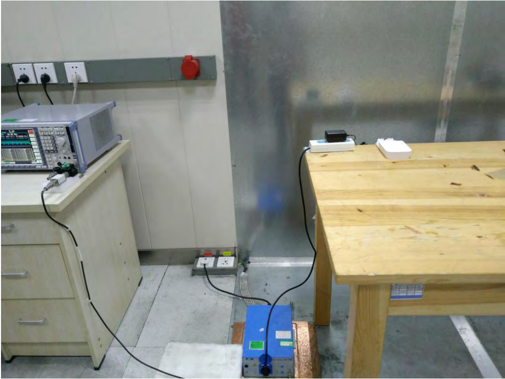
FCC RADIATED EMISSION TEST SETUP BELOW 1GHZ
