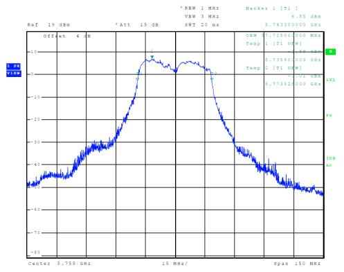
Figure 37 Plot of Transmitter Emissions (Chain 0, 5725-5850 MHz Band, 802.11n40, 99% OBW)
