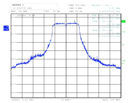
Figure 22 Plot of Transmitter Emissions (Chain 1, 5150-5250 MHz Band, 802.11n40, 26 dB OBW)
