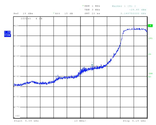
Figure 10 Plot of Transmitter Low Band Edge (Chain 1, 5150-5250 MHz Band, 802.11n40)
