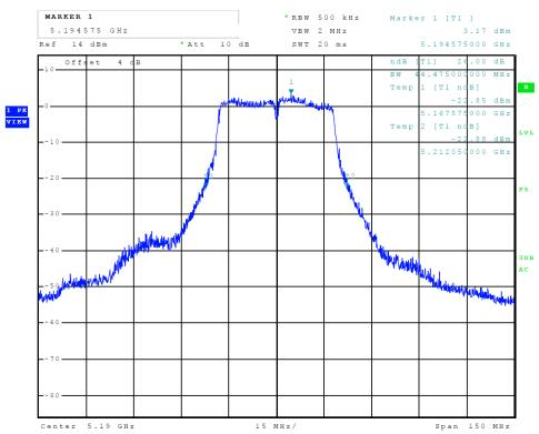
Figure 19 Plot of Transmitter Emissions (Chain 0, 5150-5250 MHz Band, 802.11a, 26 dB OBW)
