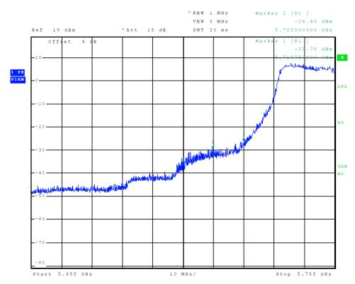
Figure 30 Plot of Transmitter Low Band Edge (Chain 1, 5725-5850 MHz Band, 802.11n40)
