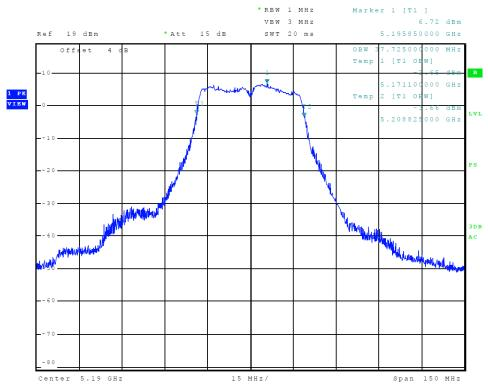
Figure 17 Plot of Transmitter Emissions (Chain 0, 5150-5250 MHz Band, 802.11n40, 99% OBW)
