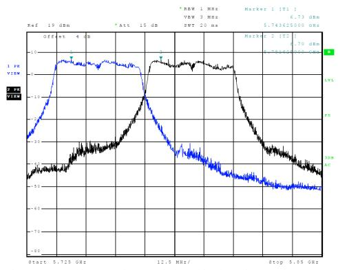
Figure 26 Plot of Transmitter Emissions (Chain 1, Across 5725-5850 MHz Band, 802.11n40)
