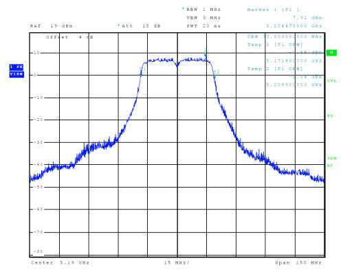
Figure 18 Plot of Transmitter Emissions (Chain 1, 5150-5250 MHz Band, 802.11n40, 99% OBW)
