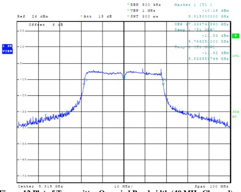
Figure 12 Plot of Transmitter Occupied Bandwidth (40 MHz Channel)
