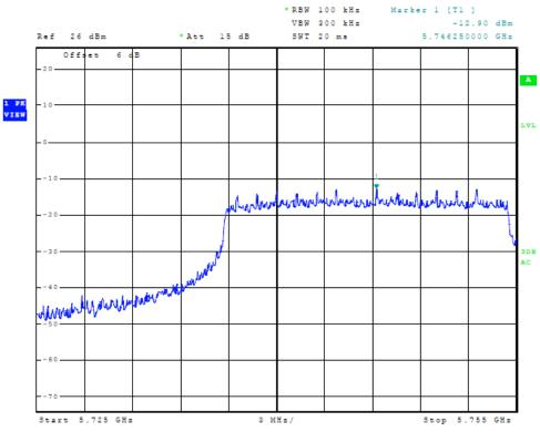
Figure 8 Plot of Transmitter Low Band Edge (40 MHz Channel)
