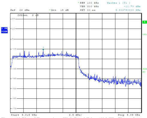
Figure 10 Plot of Transmitter High Band Edge (40 MHz Channel)
