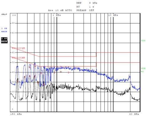
Figure 2 AC Line Conducted Emissions Line 2
