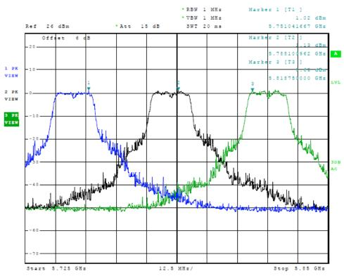
Figure 4 Plot of Transmitter Emissions (Across Operational Band, Chain 1, 20 MHz Channel)
