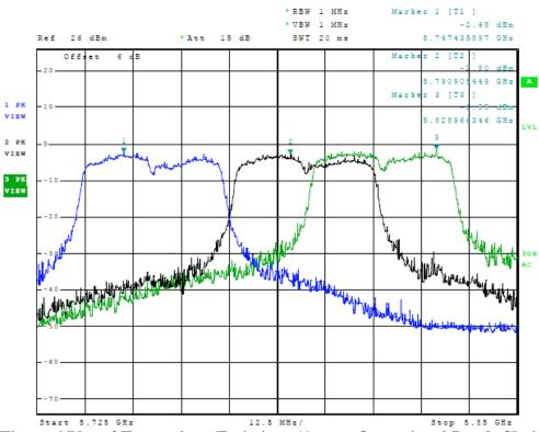
Figure 6 Plot of Transmitter Emissions (Across Operational Band, Chain 1, 40 MHz Channel)
