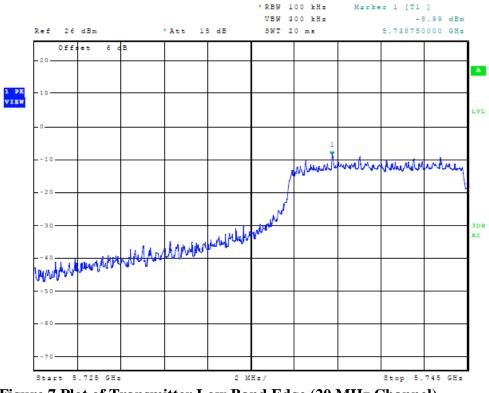
Figure 7 Plot of Transmitter Low Band Edge (20 MHz Channel)
