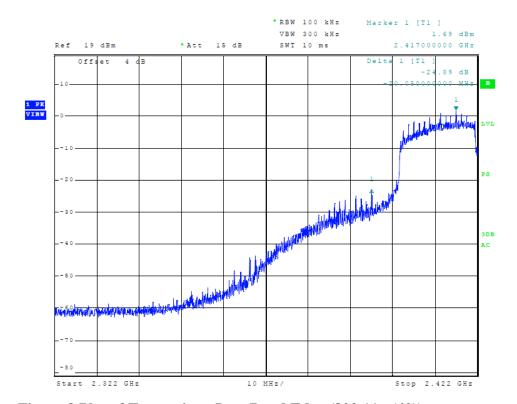
Figure 8 Plot of Transmitter Low Band Edge (802.11n (40))
