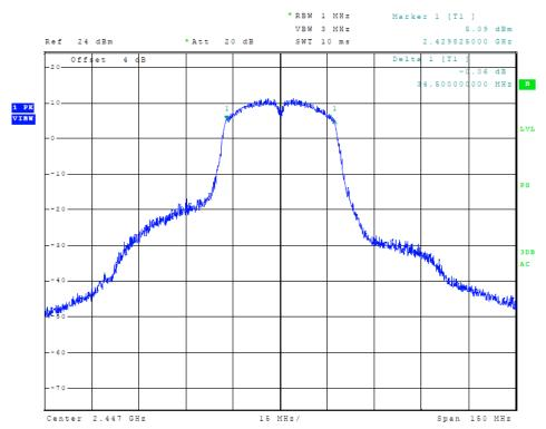
Figure 14 Plot of Transmitter 6-dB Occupied Band Width (802.11n (40))
