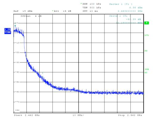
Figure 10 Plot of Transmitter High Band Edge (802.11g)
