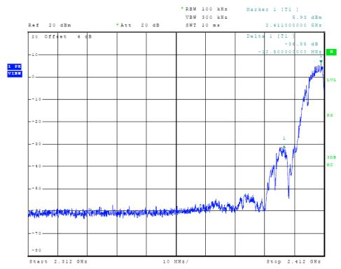
Figure 6 Plot of Transmitter Low Band Edge (802.11b)
