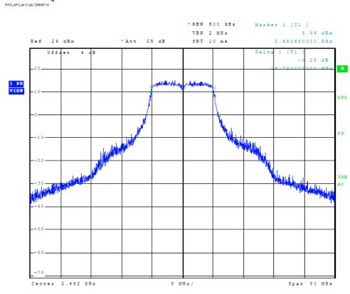
Figure 13 Plot of Transmitter 6-dB Occupied Band Width (802.11g, Chain 0)
