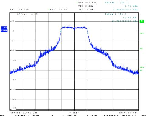
Figure 25 Plot of Transmitter 6-dB Occupied Band Width (802.11g, Chain 1)
