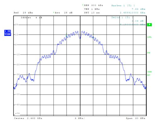
Figure 12 Plot of Transmitter 6-dB Occupied Band Width (802.11b, Chain 0)
