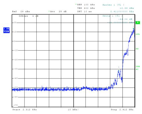
Figure 6 Plot of Transmitter Low Band Edge (802.11b, Chain 0)
