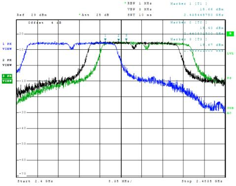
Figure 17 Plot of Transmitter Emissions (Across Operational Band, 802.11n (40), Chain 1)
