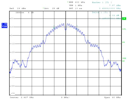
Figure 36 Plot of Transmitter 6-dB Occupied Band Width (802.11b, Chain 2)
