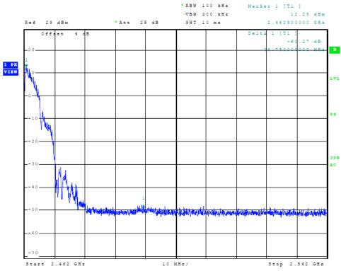
Figure 33 Plot of Transmitter High Band Edge (802.11b, Chain 2)
