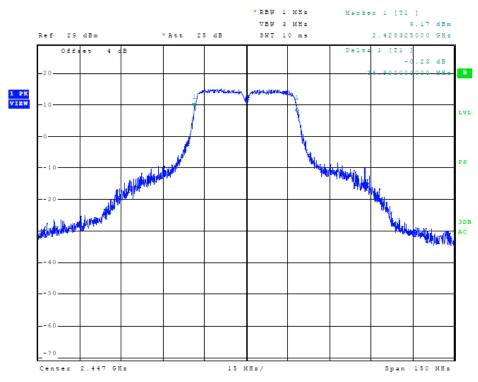
Figure 14 Plot of Transmitter 6-dB Occupied Band Width (802.11n (40), Chain 0)
