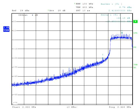
Figure 8 Plot of Transmitter Low Band Edge (802.11n (40), Chain 0)
