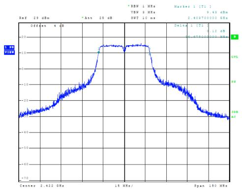
Figure 38 Plot of Transmitter 6-dB Occupied Band Width (802.11n (40), Chain 2)
