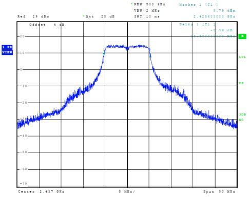
Figure 37 Plot of Transmitter 6-dB Occupied Band Width (802.11g, Chain 2)
