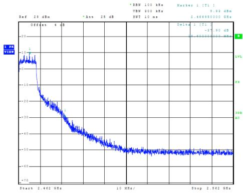
Figure 34 Plot of Transmitter High Band Edge (802.11g, Chain 2)
