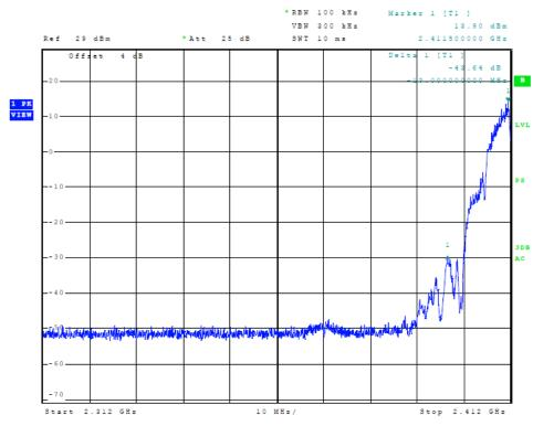
Figure 18 Plot of Transmitter Low Band Edge (802.11b, Chain 1)
