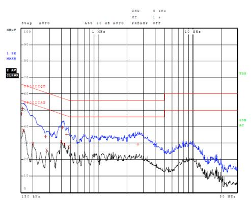
Figure 2 AC Line Conducted Emissions Line 2
