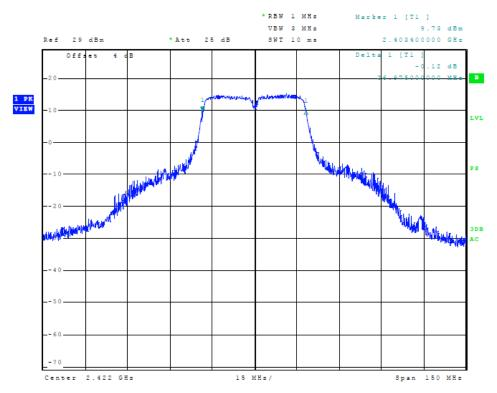
Figure 26 Plot of Transmitter 6-dB Occupied Band Width (802.11n (40), Chain 1)
