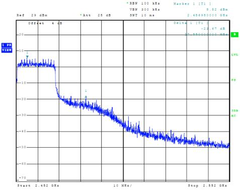
Figure 23 Plot of Transmitter High Band Edge (802.11n (40), Chain 1)
