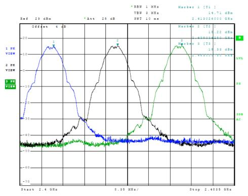
Figure 15 Plot of Transmitter Emissions (Across Operational Band 802.11b, Chain 1)
