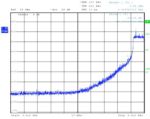
Figure 31 Plot of Transmitter Low Band Edge (802.11g, Chain 2)
