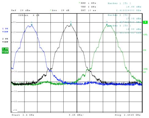
Figure 27 Plot of Transmitter Emissions (Across Operational Band, 802.11b (20), Chain 2)
