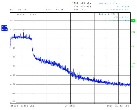
Figure 11 Plot of Transmitter High Band Edge (802.11n (40), Chain 0)
