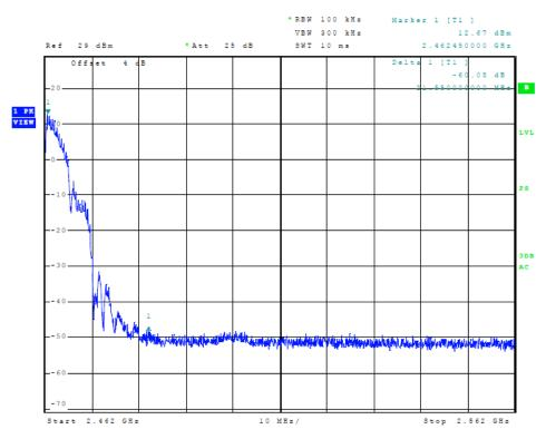
Figure 9 Plot of Transmitter High Band Edge (802.11b, Chain 0)
