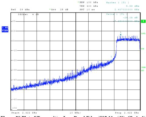
Figure 20 Plot of Transmitter Low Band Edge (802.11n (40), Chain 1)
