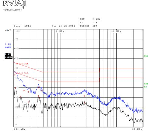
Figure 1 AC Line Conducted Emissions Line 1
