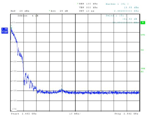
Figure 21 Plot of Transmitter High Band Edge (802.11b, Chain 1)
