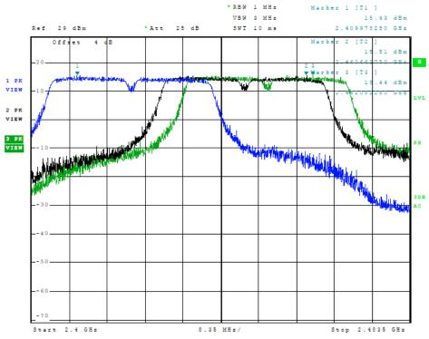
Figure 5 Plot of Transmitter Emissions (Across Operational Band, 802.11n (40), Chain 0)
