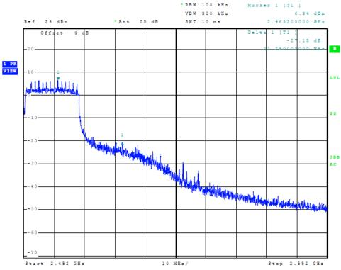
Figure 35 Plot of Transmitter High Band Edge (802.11n (40), Chain 2)
