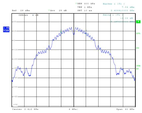
Figure 24 Plot of Transmitter 6-dB Occupied Band Width (802.11b, Chain 1)
