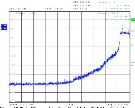
Figure 19 Plot of Transmitter Low Band Edge (802.11g, Chain 1)
