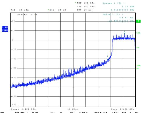
Figure 32 Plot of Transmitter Low Band Edge (802.11n (40), Chain 2)
