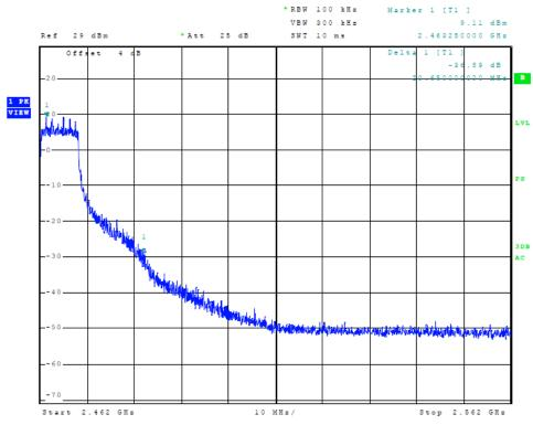
Figure 10 Plot of Transmitter High Band Edge (802.11g, Chain 0)
