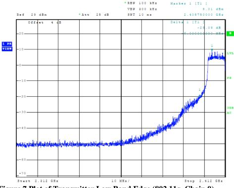
Figure 7 Plot of Transmitter Low Band Edge (802.11g, Chain 0)
