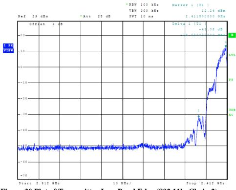
Figure 30 Plot of Transmitter Low Band Edge (802.11b, Chain 2)
