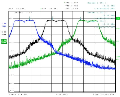
Figure 28 Plot of Transmitter Emissions (Across Operational Band, 802.11g, Chain 2)
