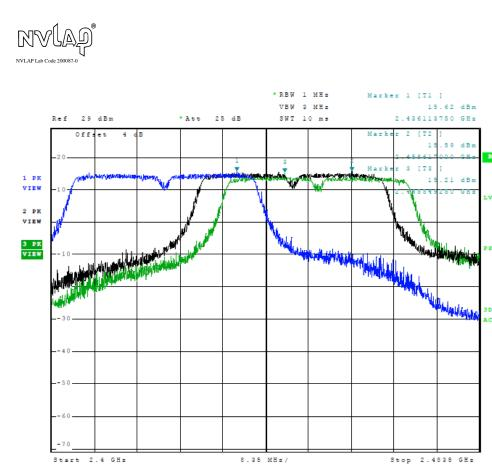
Figure 29 Plot of Transmitter Emissions (Across Operational Band, 802.11n (40), Chain 2)
