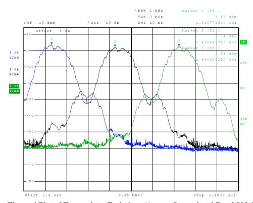
Figure 4 Plot of Transmitter Emissions (Across Operational Band 802.11b, Chain 1)
