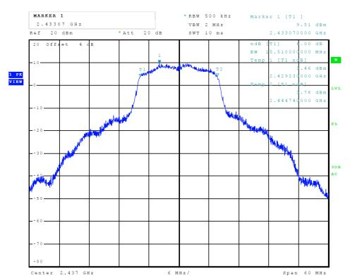
Figure 31 Plot of Transmitter 6-dB Occupied Band Width (802.11n (20), Chain 0)
