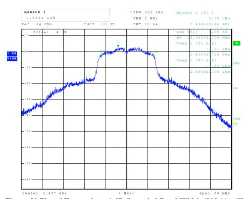
Figure 30 Plot of Transmitter 6-dB Occupied Band Width (802.11g, Chain 1)
