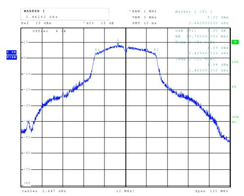
Figure 33 Plot of Transmitter 6-dB Occupied Band Width (802.11n (40), Chain 0)
