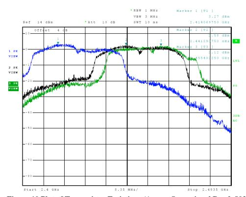
Figure 10 Plot of Transmitter Emissions (Across Operational Band, 802.11n (40), Chain 1)
