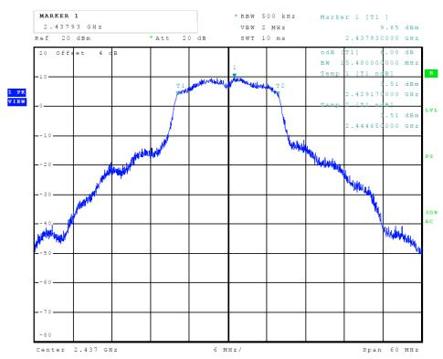
Figure 29 Plot of Transmitter 6-dB Occupied Band Width (802.11g, Chain 0)
