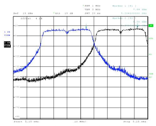
Figure 6 Plot of Transmitter Emissions (Chain 1, Across 5150-5250 MHz Band, 802.11n40)
