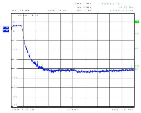
Figure 14 Plot of Transmitter High Band Edge (Chain 1, 5150-5250 MHz Band, 802.11n40)
